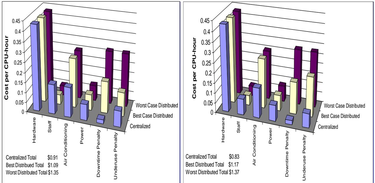
**Fig. 2.** A 2005 Indiana University TCO analysis for distributed vs. centralized HPC<sup>4</sup>
